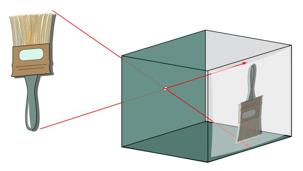
Pinhole cameras do not have lenses. There is just a small hole on one side of the box that lets light into the box. A figure is projected on the opposite side of the box.
