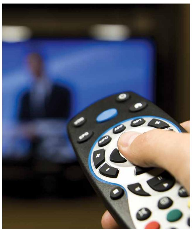
Certain wavelengths of light are invisible. We can't see the **infrared** light from a **remote control** but we can see its effect when a channel is changed.
